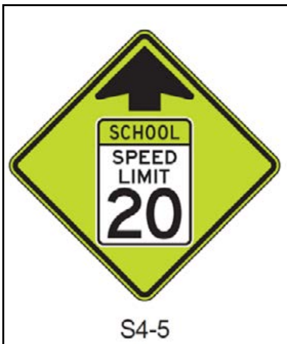
Figure 4: School Speed Limit Up-Ahead Sign Source: CA MUTCD 2014 Part 7, Traffic Controls for School Areas
