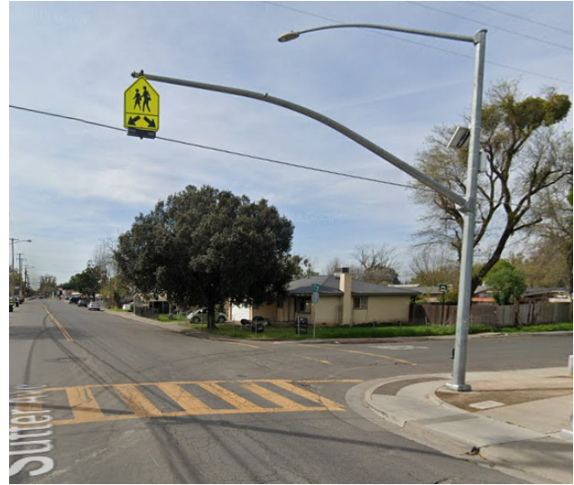
Parents and students enjoy having the RRFB signal to drivers that pedestrians are crossing, but drivers still speed through the intersection without stopping for pedestrians waiting to cross.
